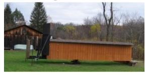
The tunnel is mounted on a pivot and is rotated every five minutes to keep a constant orientation with the sun -- directly behind the operator. Mirrors at the sides of the tunnel reflect ambient light onto the front surfaces (the 'bird approach side' of the glass, and some natural light falls on the back surface. Test materials are presented in random order and in equal frequency on the left and right side. At regular intervals, trials using
